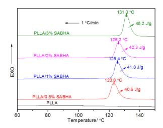
Fig. 2: Melt-crystallization process of the pure PLLA and PLLA/SABHA samples from the melt at a cooling rate of 1 °C/min.
